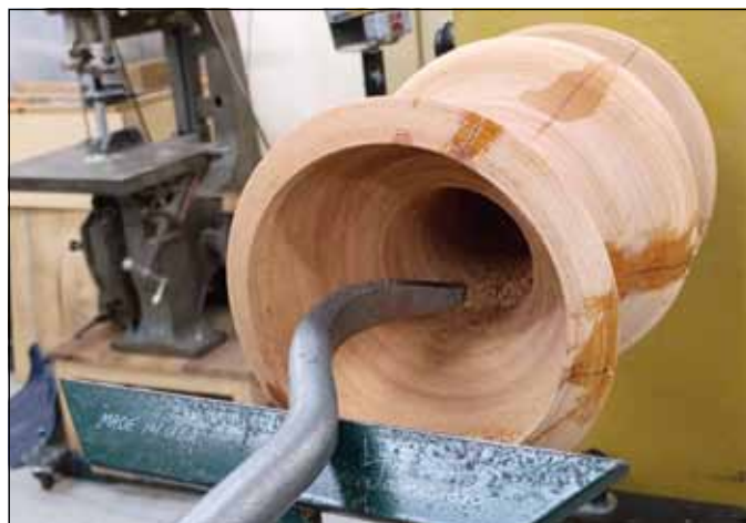
Mike used a left-hooked cutter with the lathe in reverse allowing better seeing the cut without the extreme angle over the ways.
