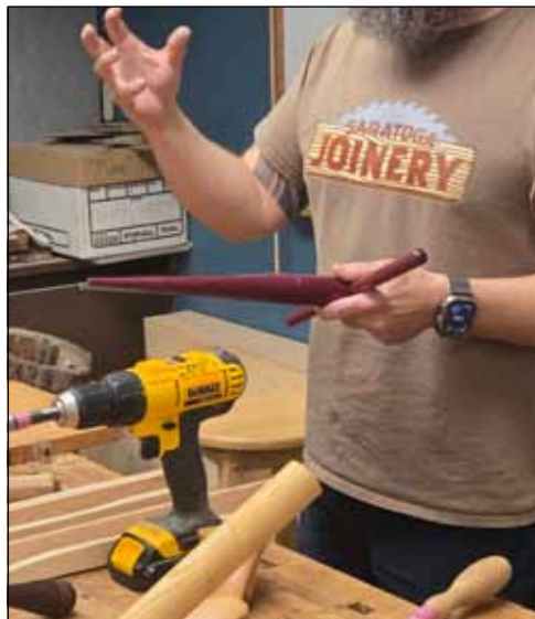
This reamer has easily removable blades for sharpening.
