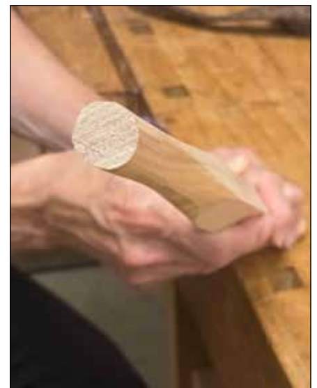
Each spindle is rounded with the spoke shave.
