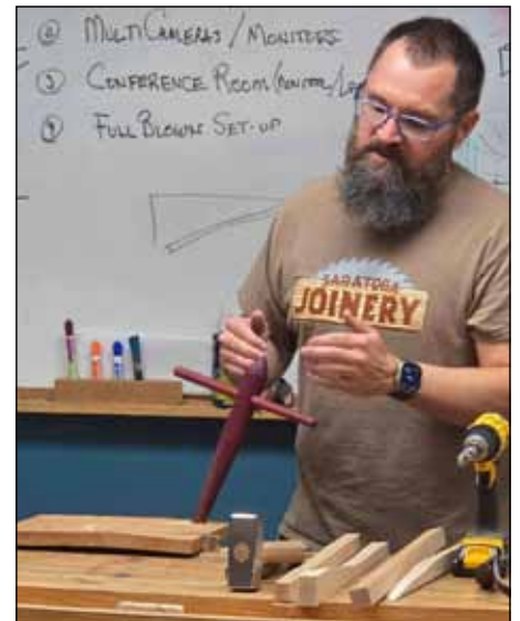
Ben cuts a tapered hole in the seat with a reamer.
