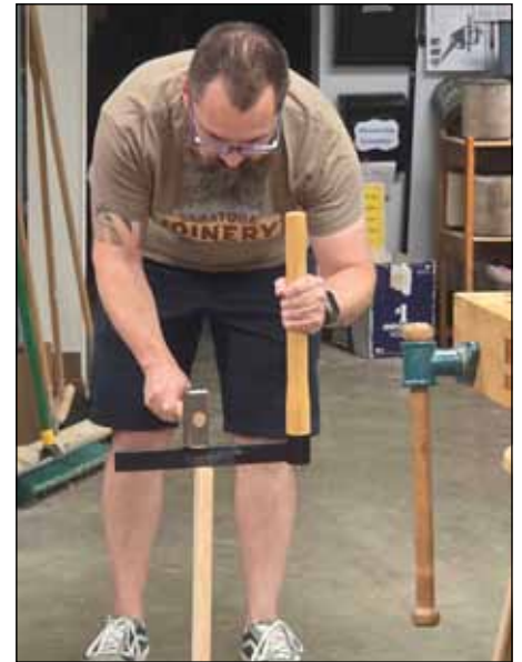
Ben uses a froe to split straight grained log.
