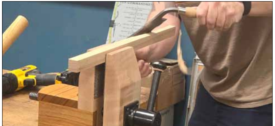
The draw knife makes quick work to make a spindle.
