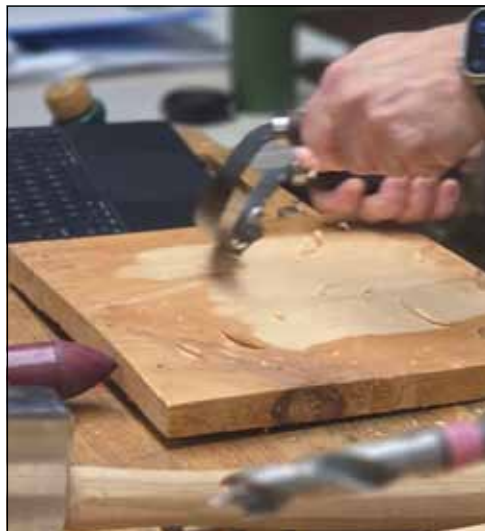
Ben uses a scorp to hollow out the seat.
