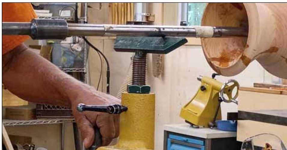
Note the locking collar for the tool rest supplied by Jamieson.
