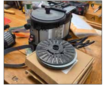
Wally's Work Sharp bench top power sharpener for plane irons and chisels.
