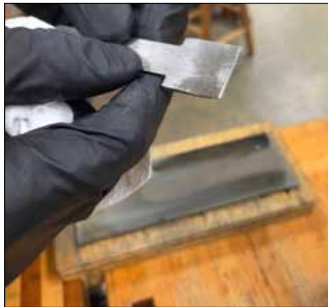
This owner polishes the back of his blade before sharpening. He uses a whet stone and leather to achieve a mirror finish.
