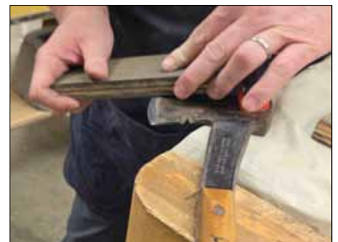
He uses sandpaper glued to a block of scrap wood.
