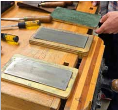
Two diamond steel plates with four grits (top side and bottom) can sharpen edges and flatten whet stones. Also leather on a board to polish the sharpened edge.
