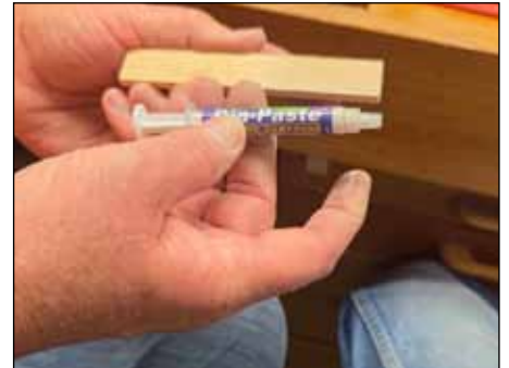
Wally demonstrates the use of diamond stone paste (1, 2, 3-micron grits).
