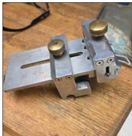
Parkis's custom-made sharpening guide, not available commercially.
