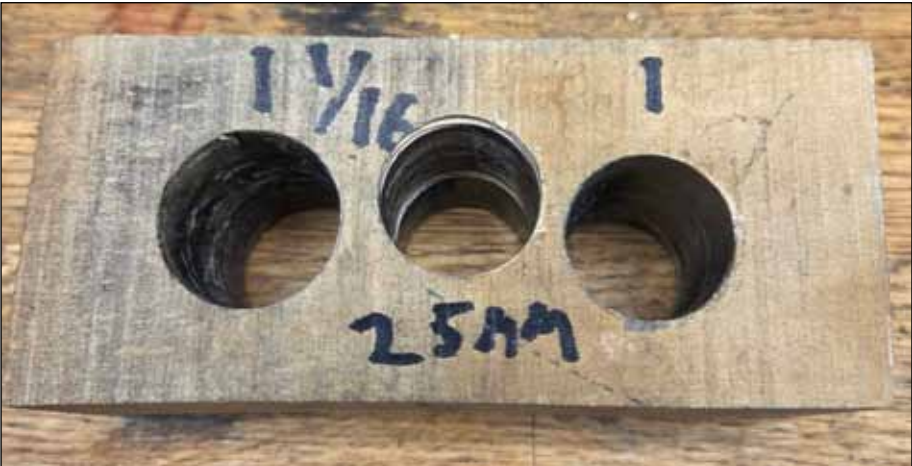
Scott's jig for measuring leg's diameter.
