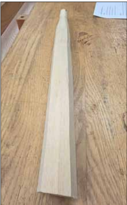
Legs should have straight grain such as this ash piece for strength.
