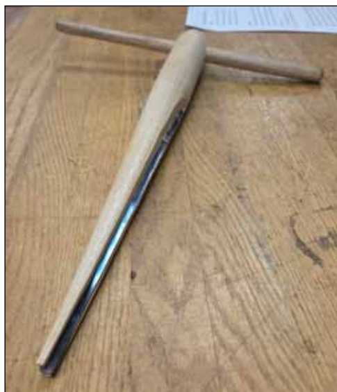
Scott's reamer's blades are sharpened to curl and dig into the sides of the mortise.
