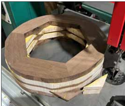
Removing the corners of the blank to prepare the piece for turning on the lathe.
