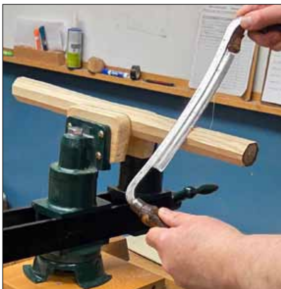
Shaping the tenon with a draw knife.
