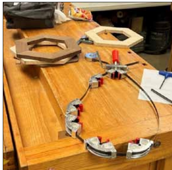
Assembled and sanded hexagons ready to be glued and stacked.
