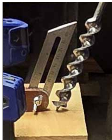
Scott lines up the auger bit with a bevel gauge.
