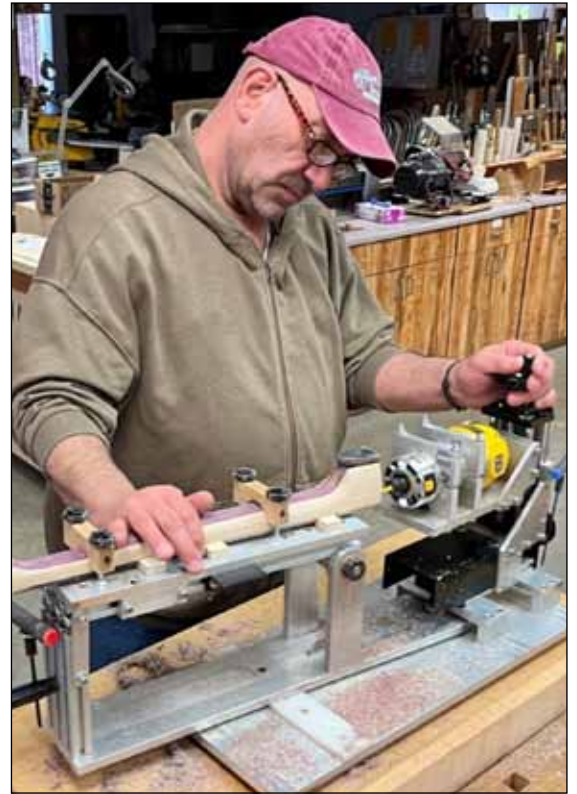
Steven uses Ray's neck radiusing jig.
