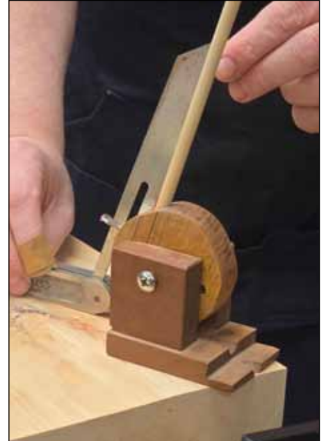
The bevel gauge allows adjustment of the rod's angle.
