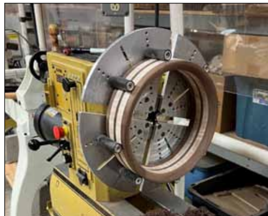
Mark's finished banjo pot ready to be dismantled from the Cole Jaws (Peruvian Walnut, Hard Maple).
