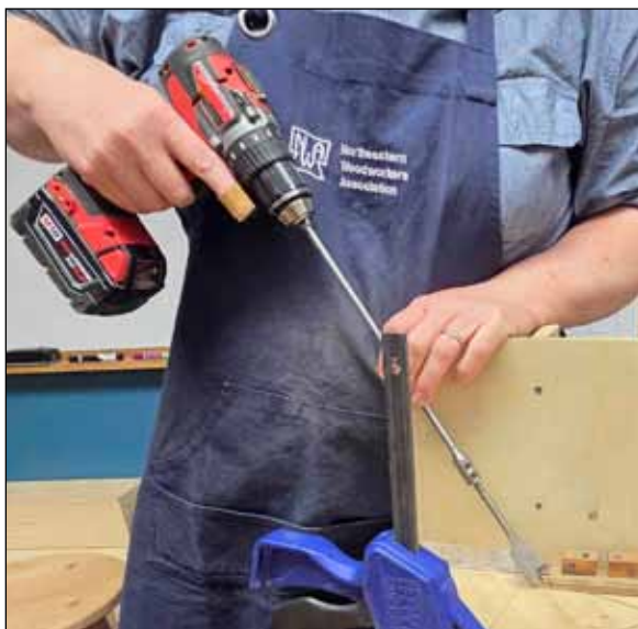
Peter Gilbert's jig design holds the drill bit's extension at the desired angle.
