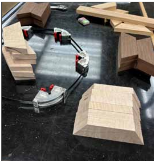
Stacks of trapezoids ready to be glued together to become the pot of the banjo (Peruvian Walnut, Hard Maple, Hickory).
