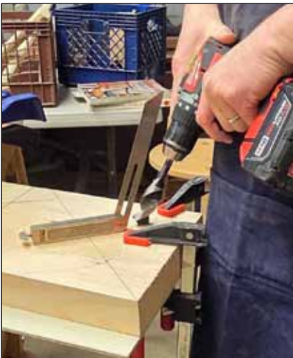
Using a bevel gauge to keep the correct angle of the drill.
