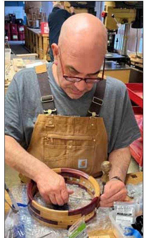
Steven installs the hardware onto his completed banjo pot (Purpleheart, Hickory, Maple, Yellowheart).
