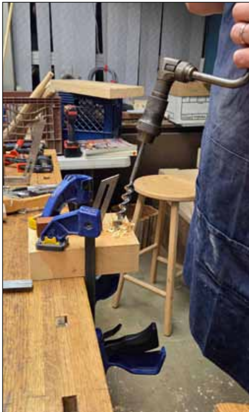
First method of hole drilling is with a brace and auger bit.
