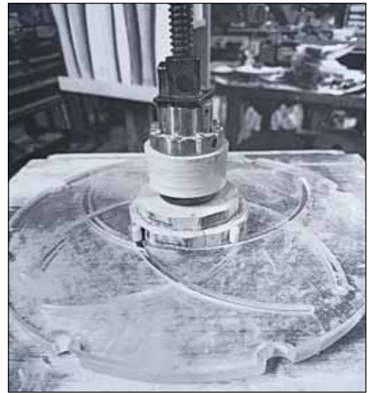
A Longworth chuck holds the rings in place within the stomper.
