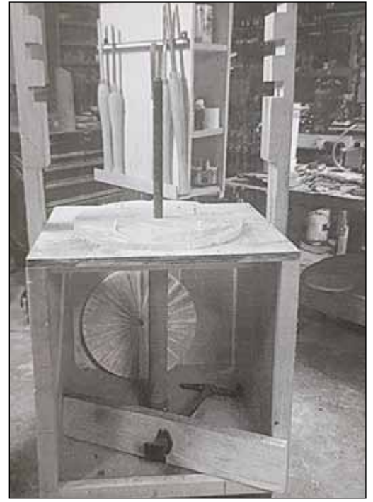
Each succeeding ring is glued together in a spring-loaded device: the stomper.
