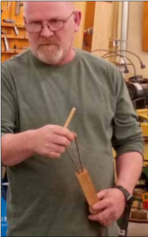
As the rings – or editions – are glued, Dave joins them with a shop-made clamp.
