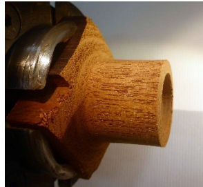
Figure 33. Jam chuck recess cut.
