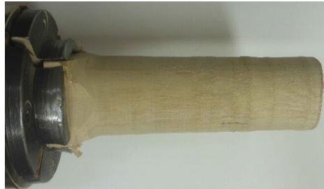
Figure 2. Billet rounded, check for defects.
