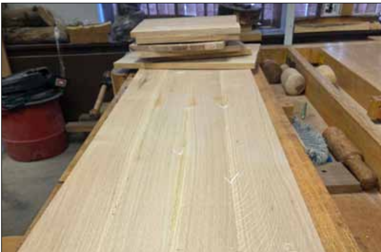
Although its boards are precisely planed to the same thickness, there is movement that frustrates the glue up.
