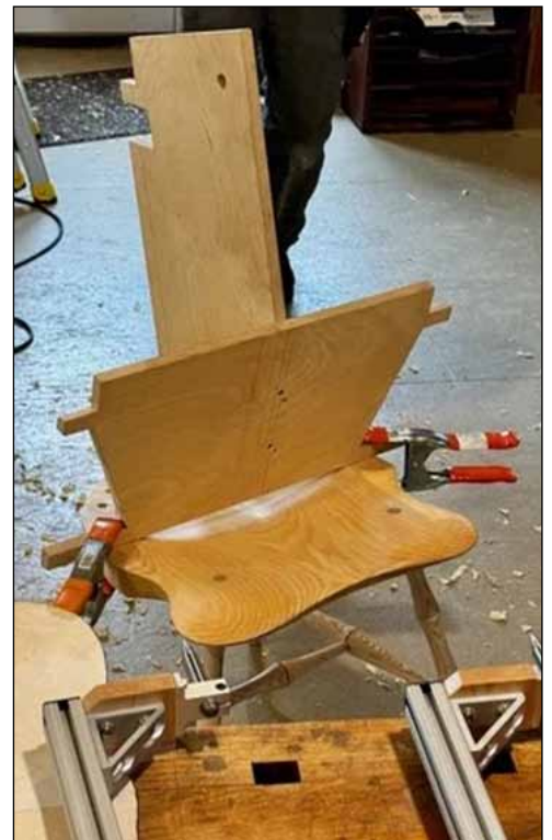
Fixture to hold the arm bow in place while drilling mortises.
