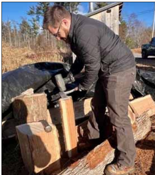
Splitting out spindle stock from white oak logs.
