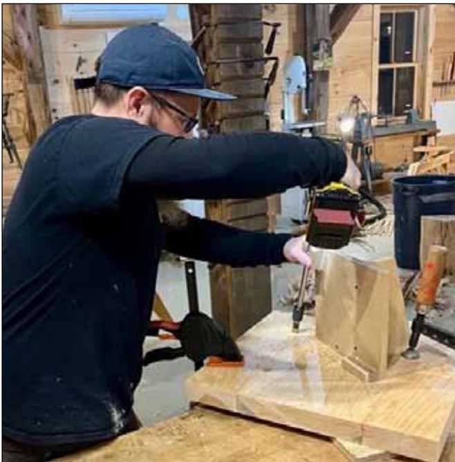
Drilling seat mortises with a drilling fixture.
