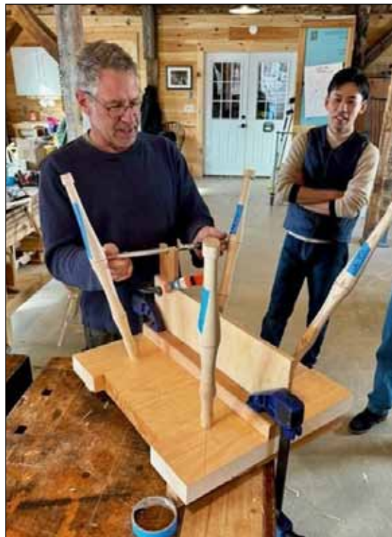
A couple pieces of plywood and some clamps make drilling leg mortises a breeze!
