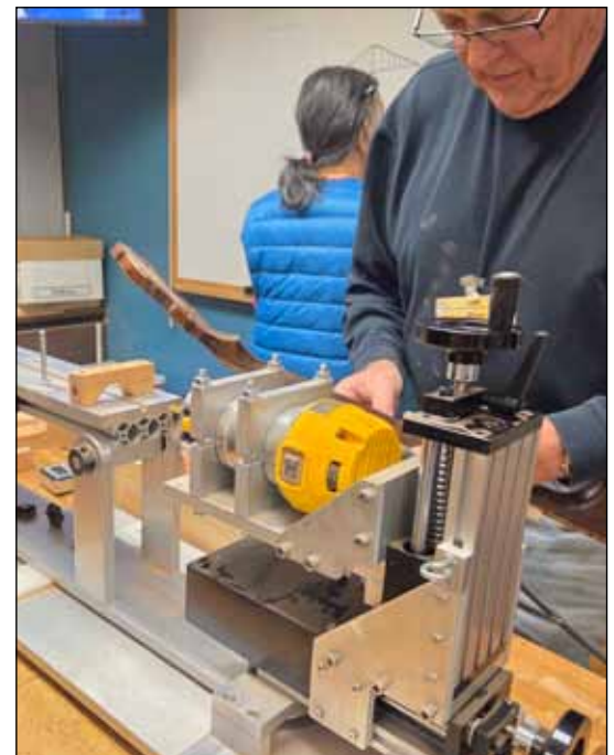
Ray's custom made machine to cut the guitar neck to the pot
