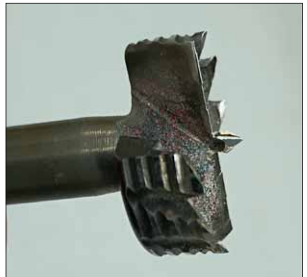
A Famag drill is recommended for creating the through hole in the blank
