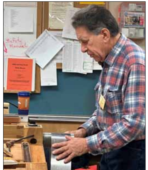
Eric demonstrates heat bending techniques for forming guitar sides
