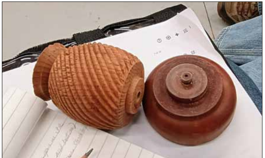
A jam chuck with a tenon is used to finish the top of the peppermill
