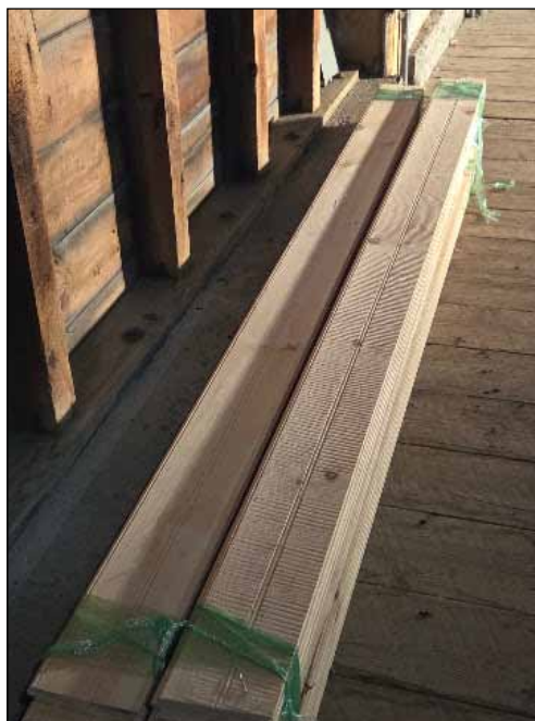
Stock planed, texturized, and fitted tongue and groove boards
