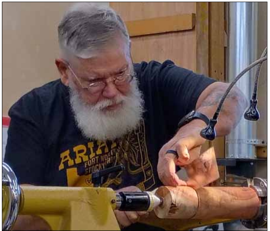
Doug cuts off the top of the peppermill blank with a thin kerf saw
