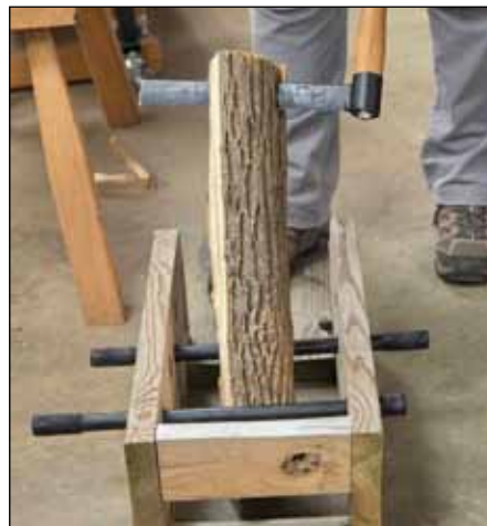
The froe follows the grain, and Scott will use a hatchet to keep the wood from springing shut.
