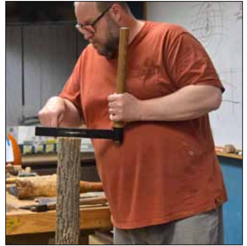
The froe removes the bark and quarters the log
