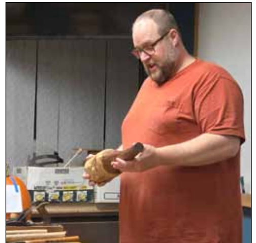
The froe club is used to strike froes and hatchets. Never use a metal hammer.
