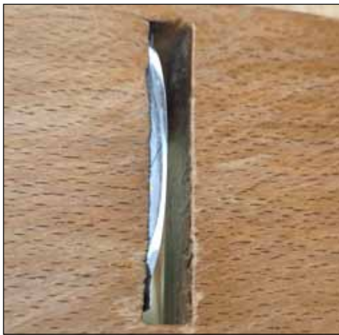
Note the wide mouth makes aggressive quick cuts
