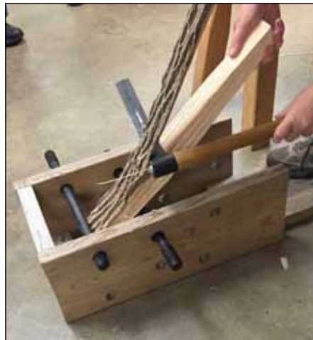
This box with adjustable black bolts secures the wood while Scott trims the bark off one quarter
