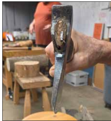
Kent Pattern Hewing Axe. Note the single sided beveled edge.
