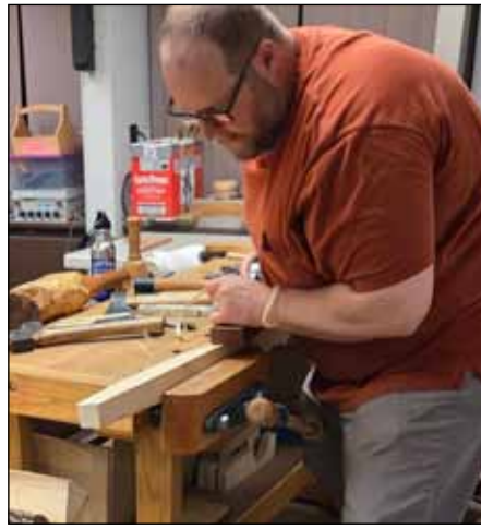
He planes the blank with a wide mouth wooden plane that cuts thick shavings
