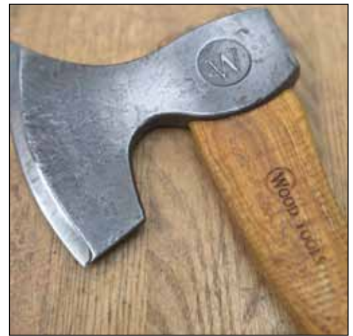
The Sheffield Axe from Wood Tools. It is a carving hatchet in the Scandinavian style made in England.
