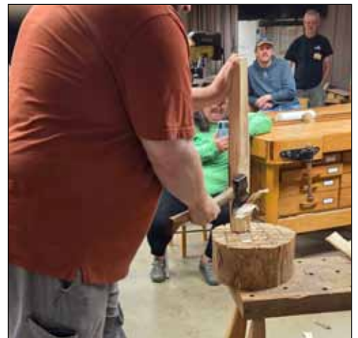
Scott trims the leg with a very sharp hatchet
