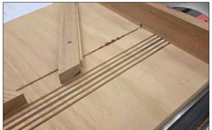
Saw blade set at 4 millimeters
