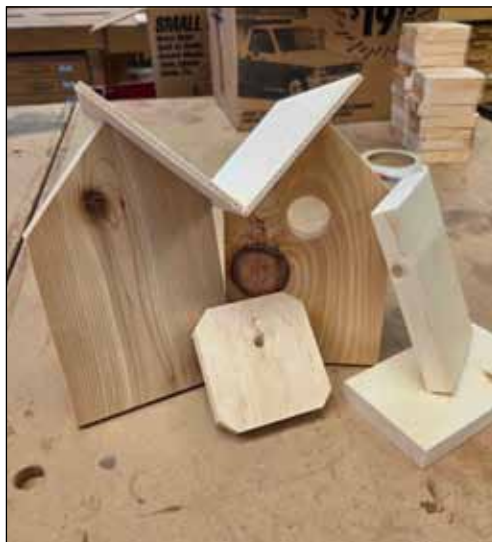
One birdhouse parts with predrilled holes for nails
