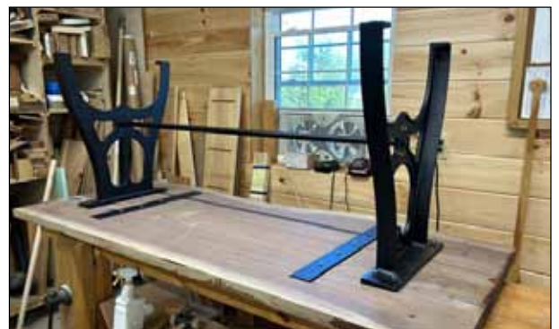
Legs and are stretcher are mounted
