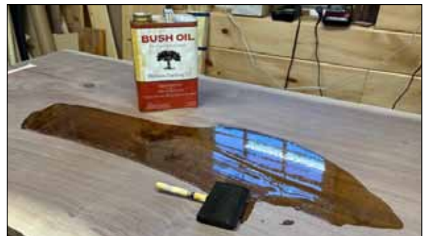
After sanding to 400, Bush Oil is liberally applied
