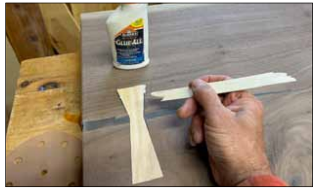
Epoxy and butterfly joints used to secure the end cracks
