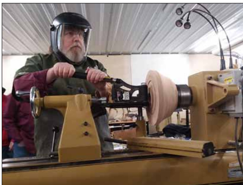
Note the Woodcut broad platform and connection to tailstock
