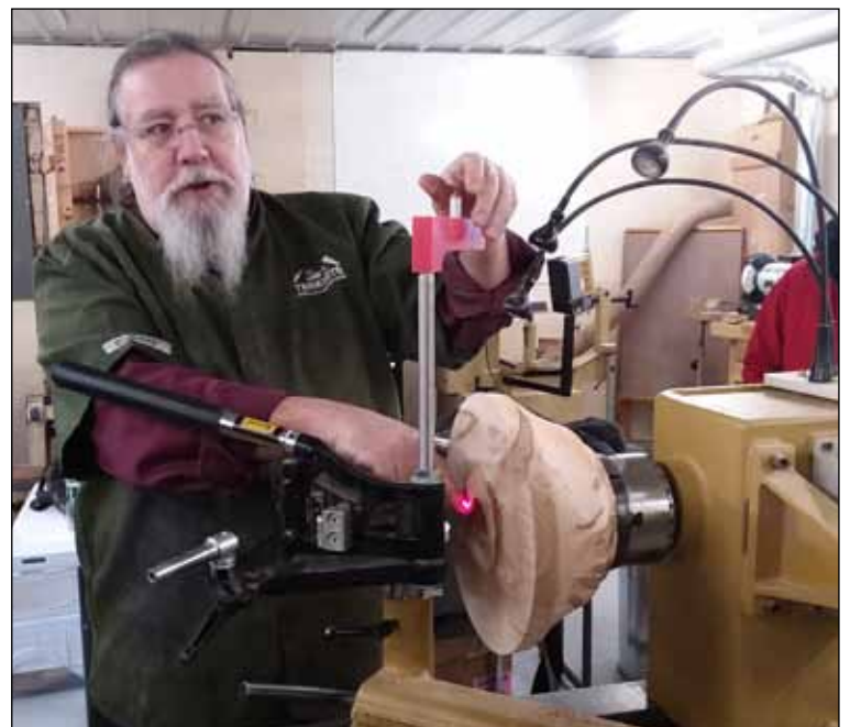
Stan Pressner shows how the laser guide works on the Woodcut Bowl Saver
