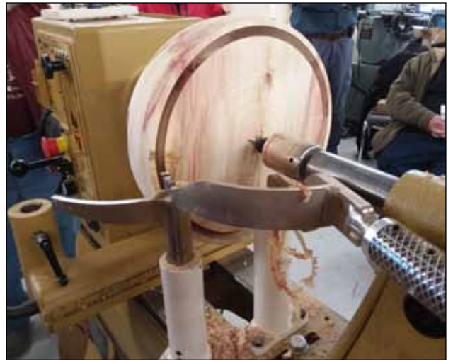
Oneway Easy Core system showing cutter arm and "finger" rest for the cutter. The cutter slides over the finger rest and can be inserted into the kerf
