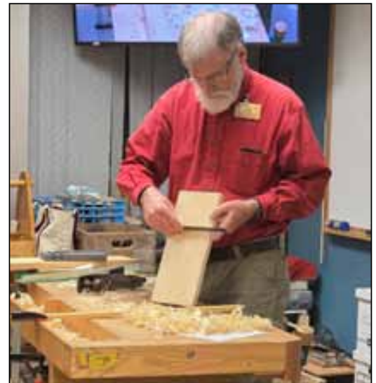
Doug shows the iterative process of planing and checking for flat
