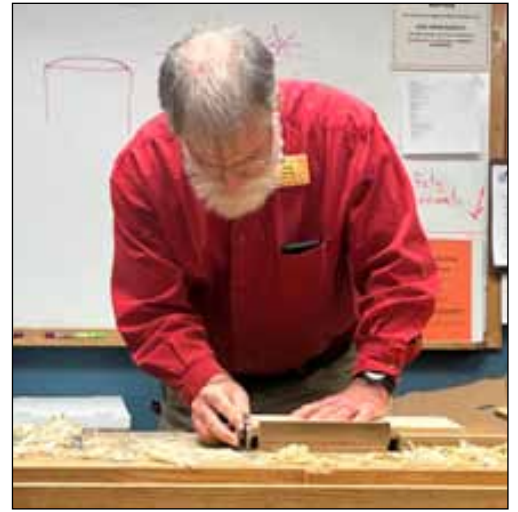
Doug crosscuts to final thickness and finishes the surface with a low angle block plane and shooting board
