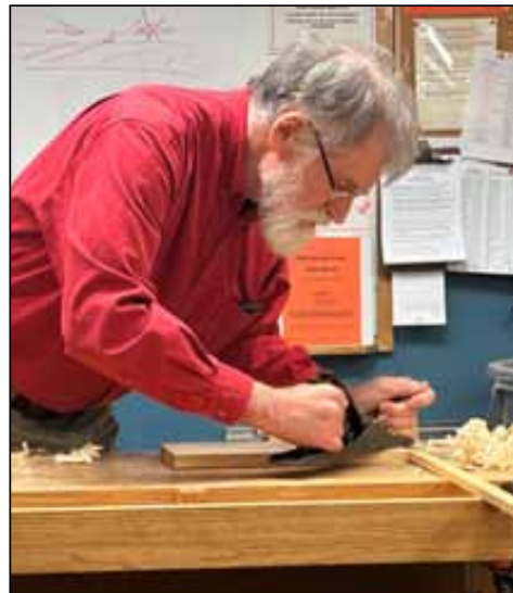
Doug shows the iterative process of planing and checking for flat
