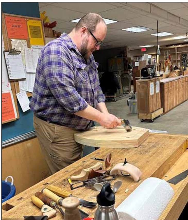
Initial use of the scorp for rough shaping of a Windsor chair seat
