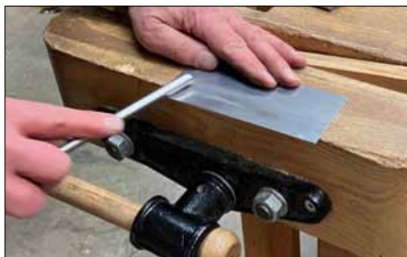
Drawing out edge of card scraper in preparation for setting the burr
