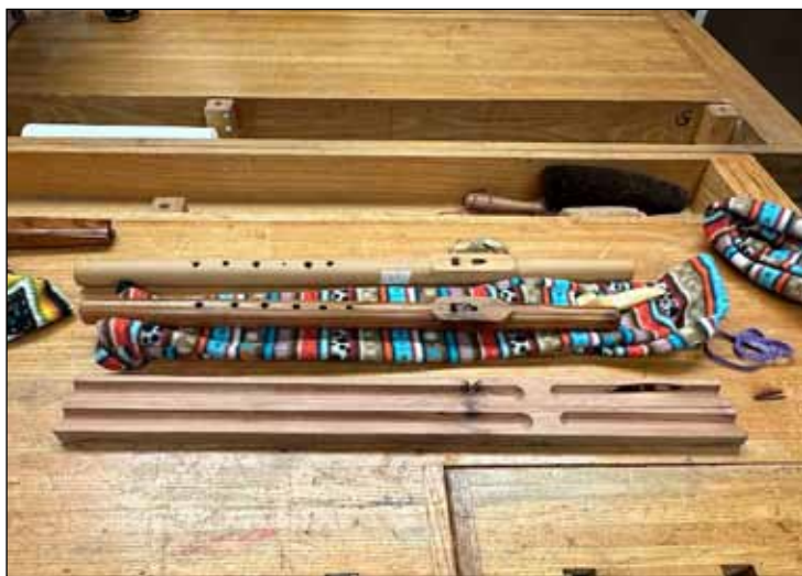
Native American style flute sound chamber is formed on the board (front), then glued up to form the flute (behind.)
