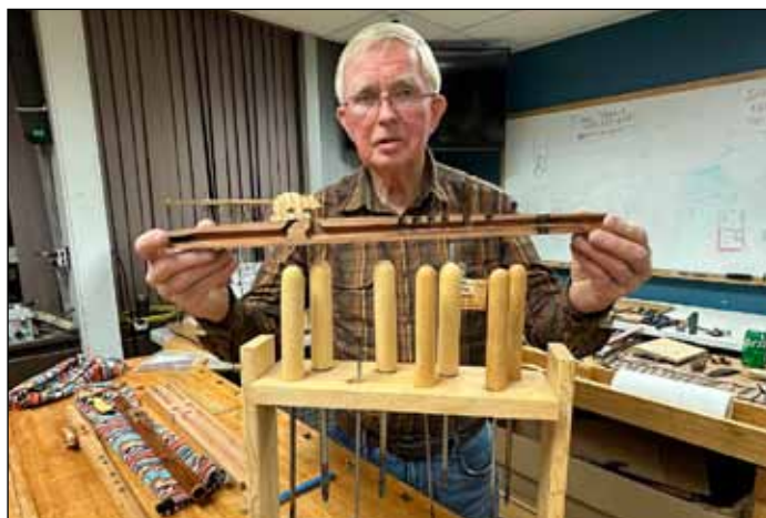
Jon Hedman drills pilot hole for finger hole according to the map, then uses burning stick to enlarge it to the appropriate size. Burning stick is forgiving, easily can make minor adjustment for the finger holes.
