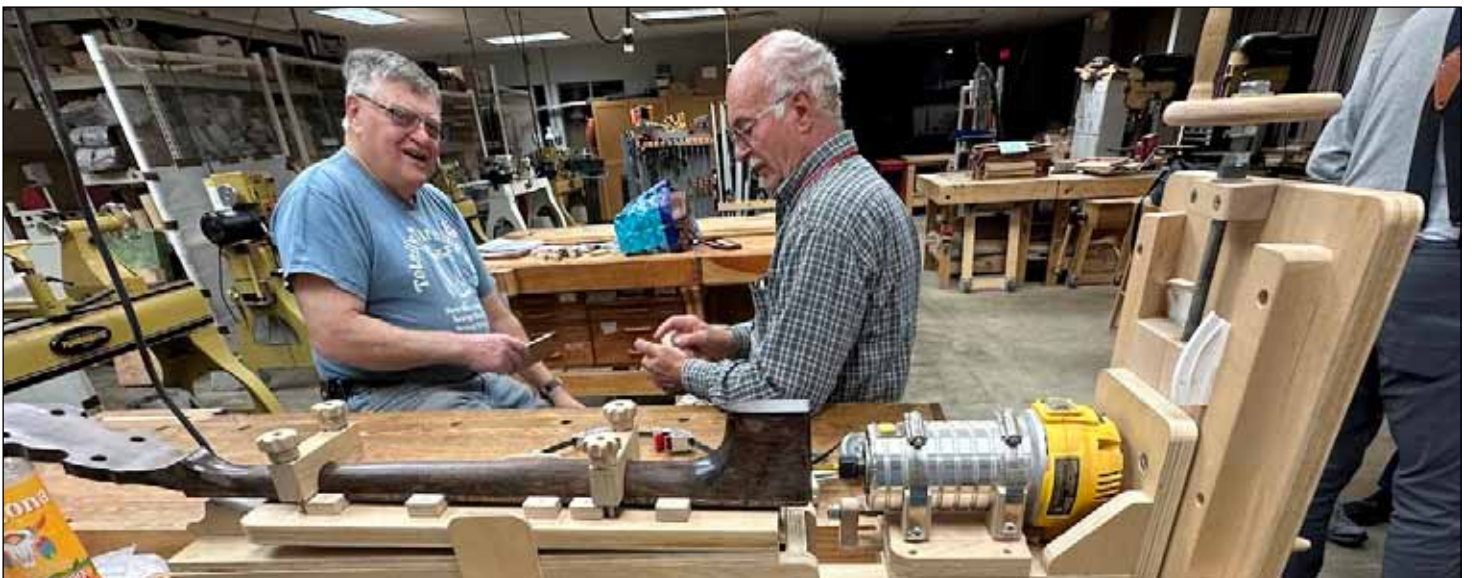
Jig designed by John Michne (past NWA President and current Newsletter Editor). Horizontally mounted router shapes the neck end to match banjo body.
