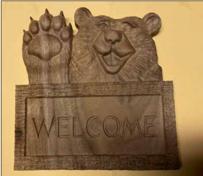
Ernie & Diane Balch CNC routed the Welcome Bear sign from walnut. It measures 8" wide x 9" high x 1 1/8" thick. Diane will apply Tru-Oil Gunstock Finish.
