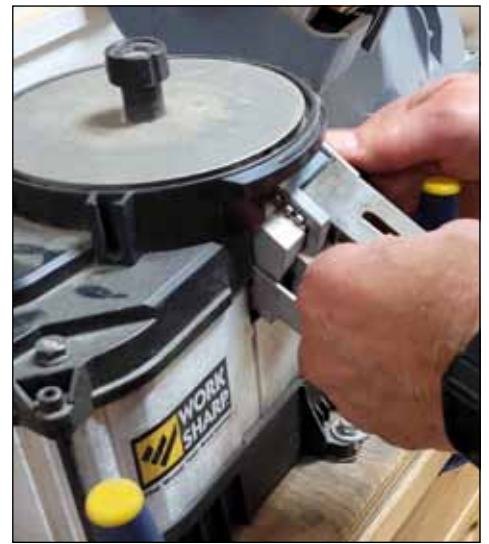
The Work Sharp is a motor-driven disk with multiple grits and adjustable bevel angles. Our shop has one you can try. It retails for about $240.
