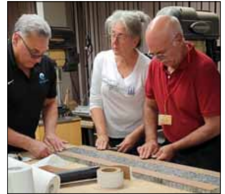
Three participants polish the backs of their chisels to a mirror finish. This is a tedious process but needs to be done only once.
