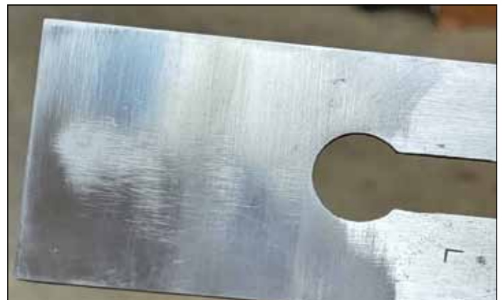
This iron is polished ¼ to ½ inch from the edge and is ready to be sharpened.
