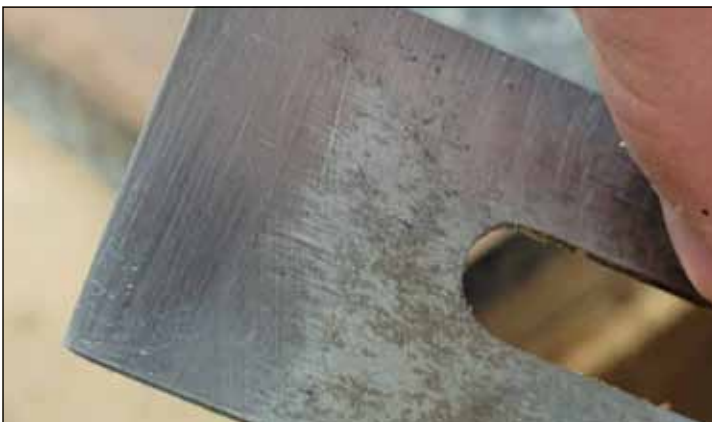
Scratches reveal what is not yet flat on this plane iron.
