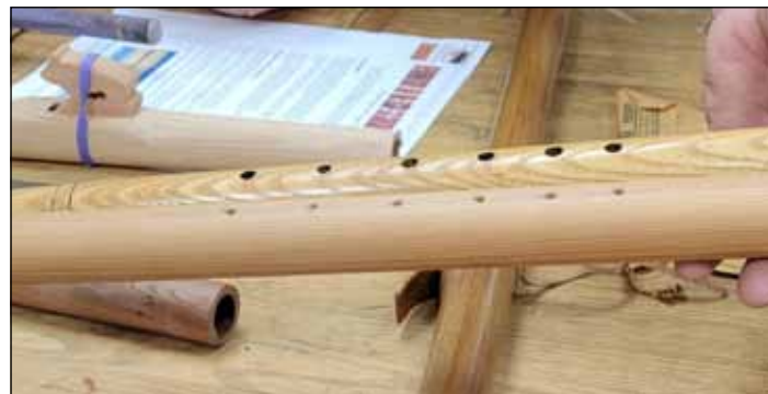
Two flutes, one tuned, the other with drilled holes aligned
