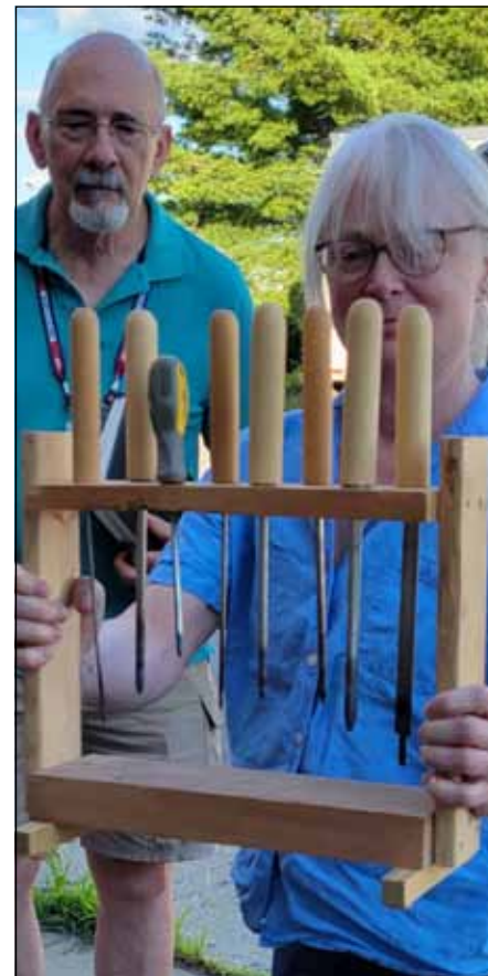
Rods are used to burn holes of specific diameters
