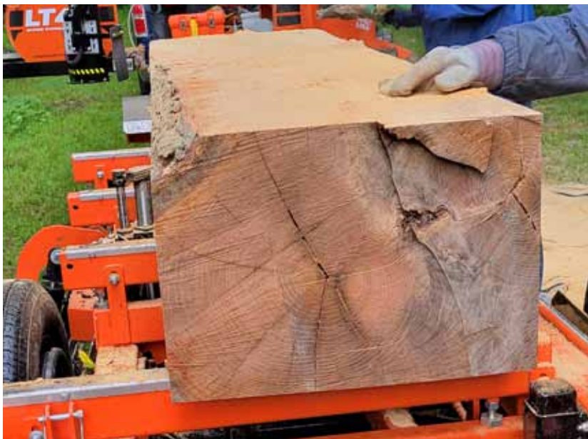
The log is square to slice about 14 boards.
