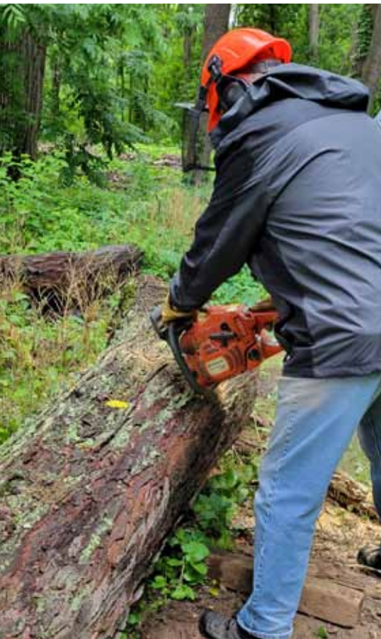
Ray Puffer chainsaws log's irregularities, so it will sit safely
