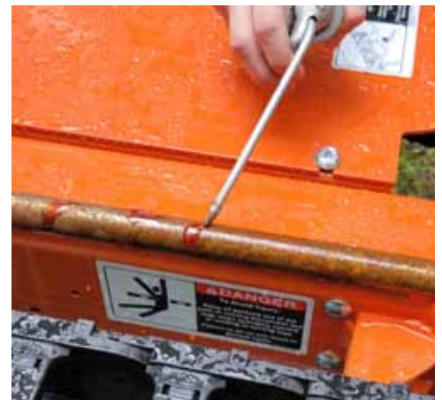
The Wood Miser's rails are oiled with ATF oil
