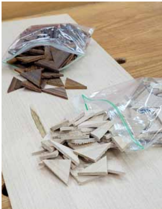
Splines or feathers for box corners
