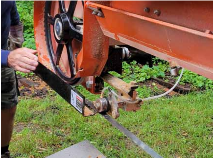
Rick Bird helps Lee install a new blade
