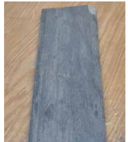
Gabon ebony could be steamed bent for the sides
