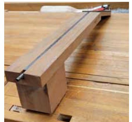
A steel guitar neck with truss rod mahogany
