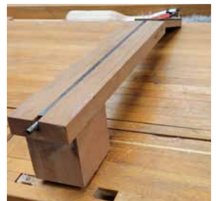
A steel guitar neck with truss rod mahogany
