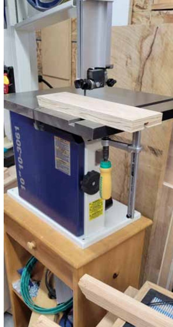
The smaller band saw with Paul's invented guide
