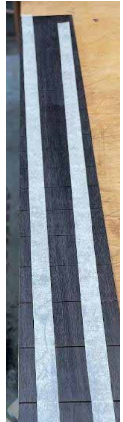
The fingerboard edge is tapered according to the posterboard template.
