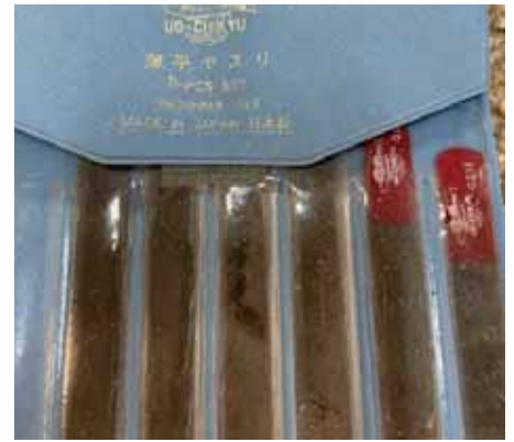
Thickness files for making grooves in the nut
