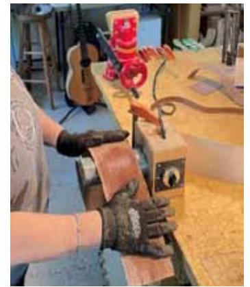
Bending sides with water and heater.
