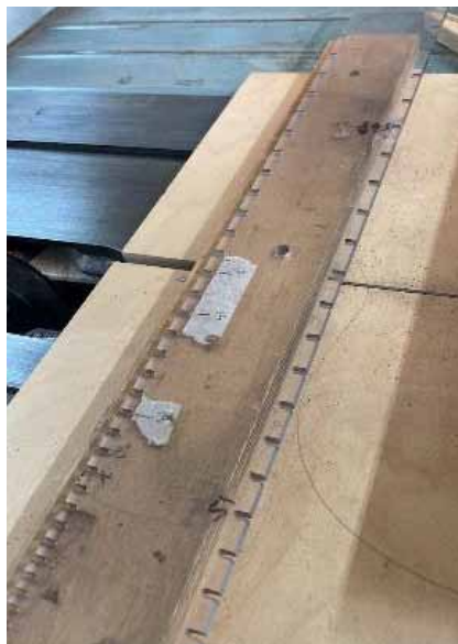
Fret board material is attached to jig with 2 sided tape.
