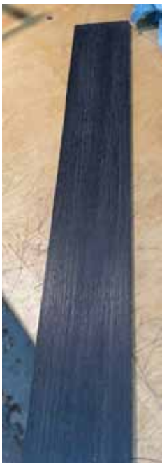
Fret board material is attached to jig with 2 sided tape.
