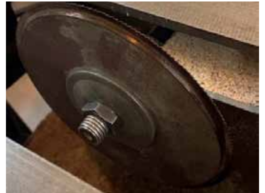
Pin on fence fits into each slot in turn then it is passed over the specialty blade.
