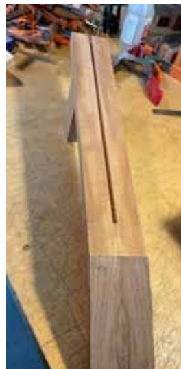
A groove is routed for the tension rod that will be inserted into the neck.
