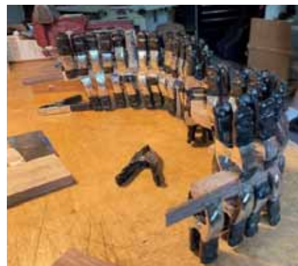
The linings are glued to the sides of the guitar with more Titebond and lots of clamps.
