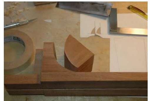
My first heel cut on the neck block. This is done on the bandsaw
