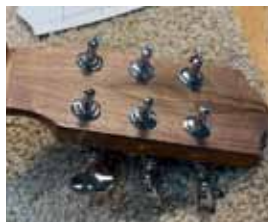
Holes are drilled at the correct spacing to allow for the machine heads to turn without interference.
