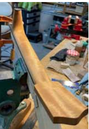
After much rasping, card scraping, sanding the final neck shape has been accomplished.
