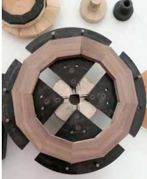
A larger ring held fast in jumbo jaws for flattening the face
