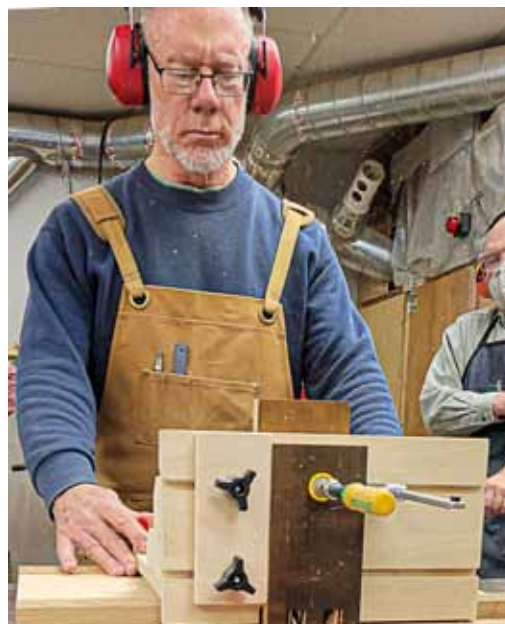
He cuts the spaces between fingers with multiple, precise passes
