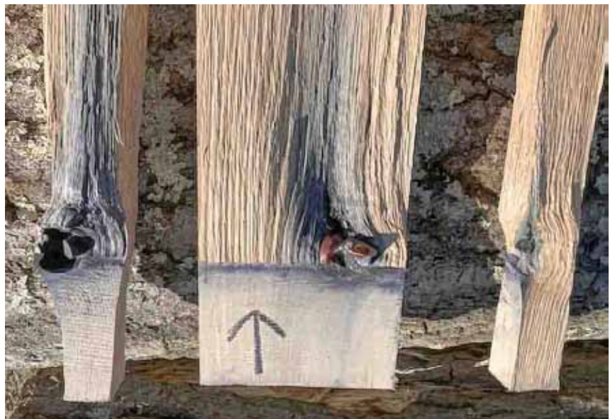
C-2 shows the insulator in the log and the pieces that were covering it in photo C-1
