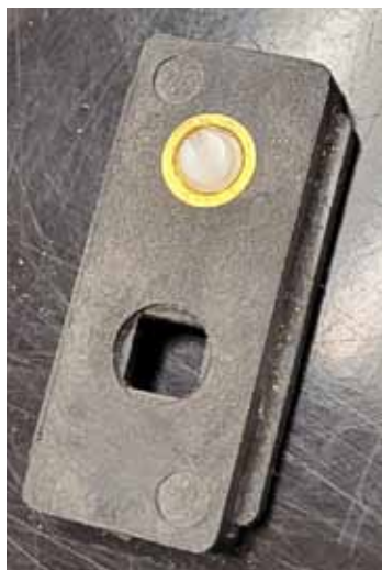
Stop used on table saw's miter groove
