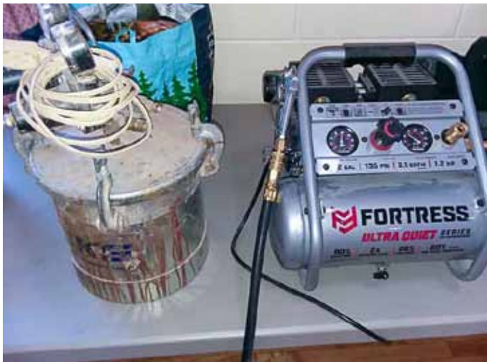
Pressure pot and compressor used for resin casting
