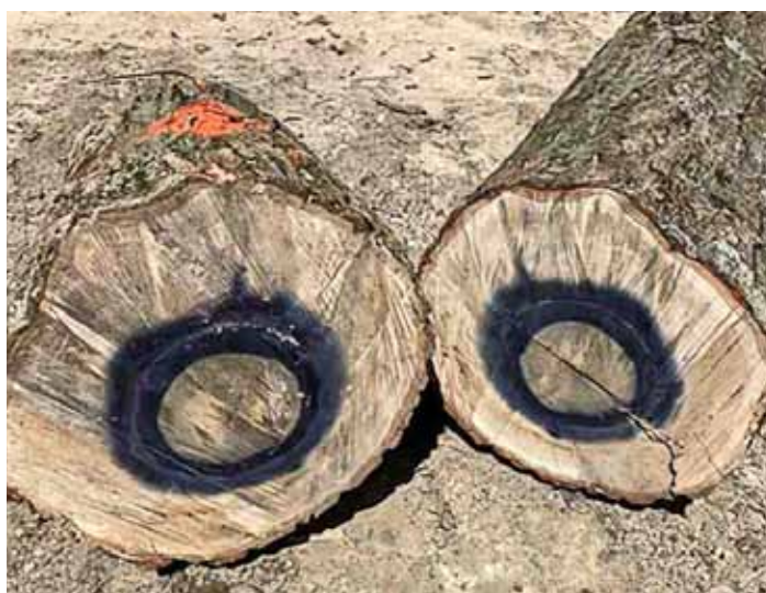
B-2 The bluing on the end of the log is one foot from the metal
