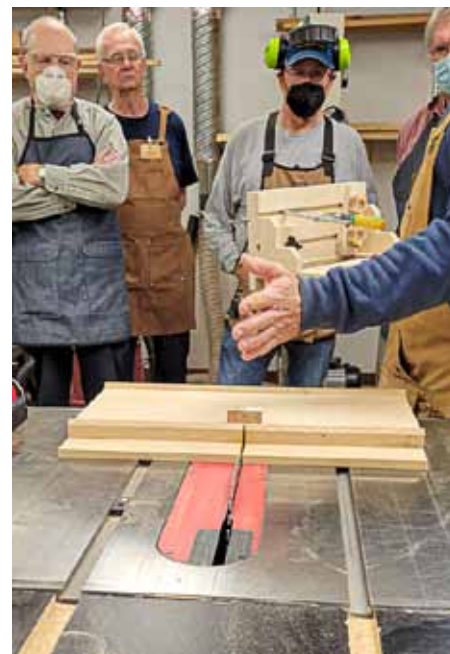
Paul points to two blocks which guide the placement of the jig on the sled
