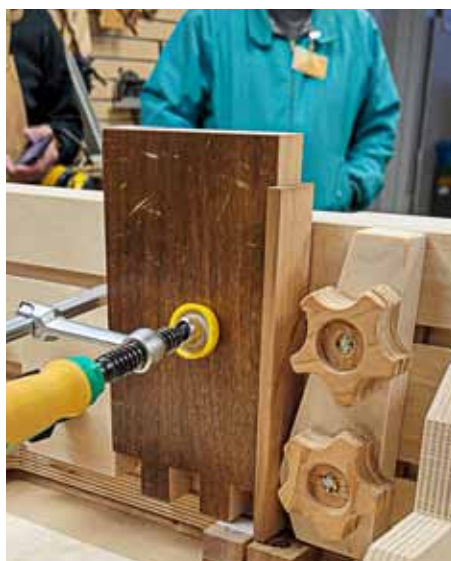
Complementary fingers on the jig's back side guide the cuts
