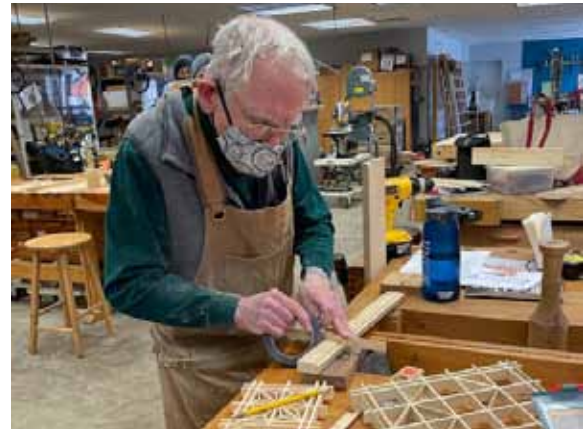
The panel frame is notched with a fine-tooth saw
