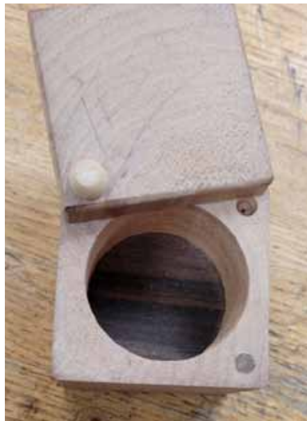
The interior shows hinged lid with earth magnet
