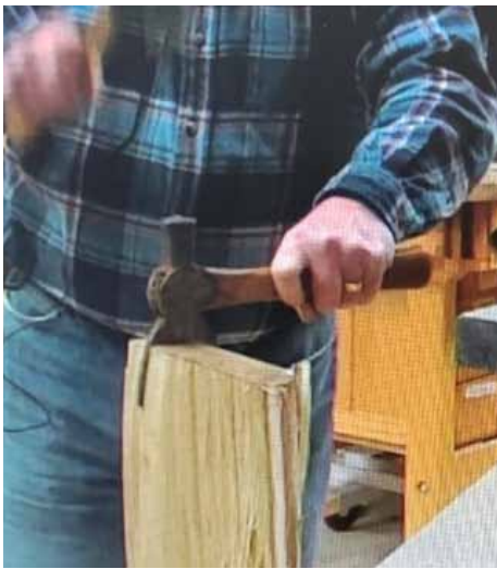
Riving 8" pegs from stock locust with shake froe
