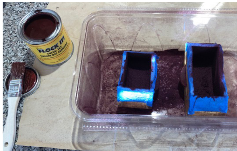
The drawers just after applying the Flocking fibers.
