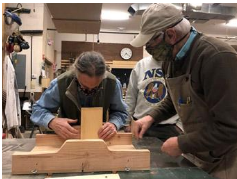
Cutting sides of dovetails on the table saw
