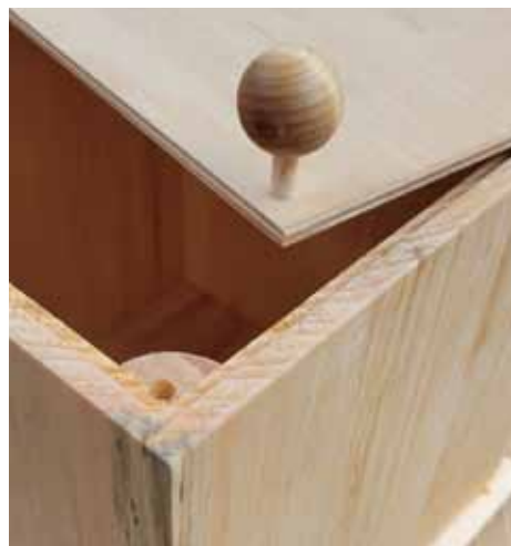
Bottom secured with pins
