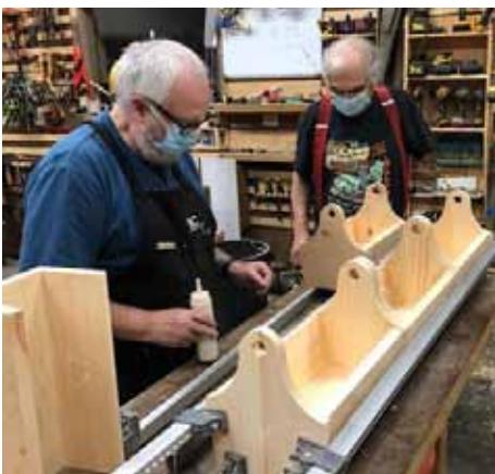
Gluing up ends to previously glued sides and bottoms
