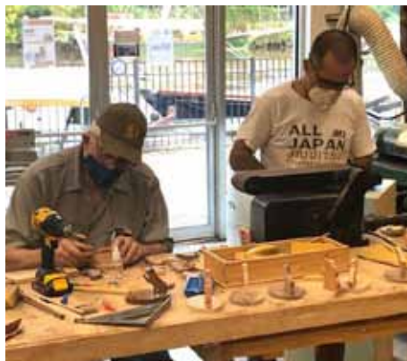
Assembly of figures to base. Each figure was cut out on the scroll saw
