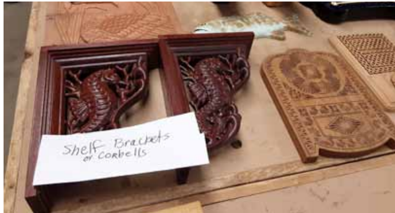
CNC items made by Ernie Balch - Jatoba wood, 2-sided Seahorse shelf bracket/corbel
