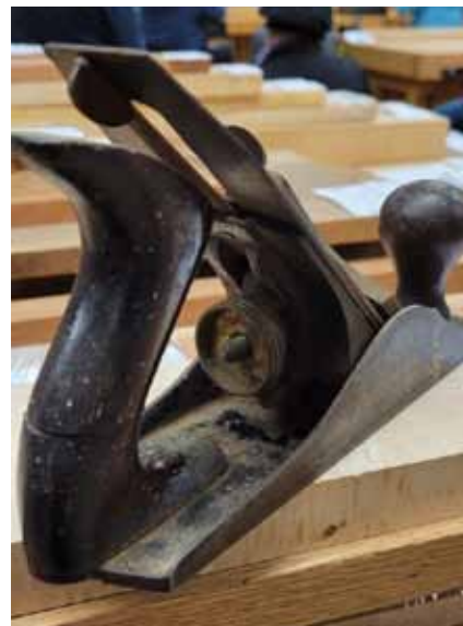
Restorable plane with cracked tote, a film of rust, and small pits
