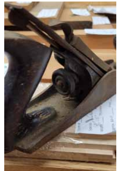
Plane with Bakelite adjuster which replaced brass ones during WW II
