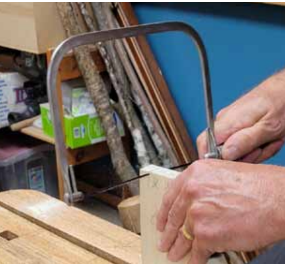
Chuck cuts waste between pins with coping saw.
