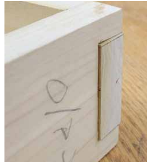
The proud dovetail will be trimmed off last.
