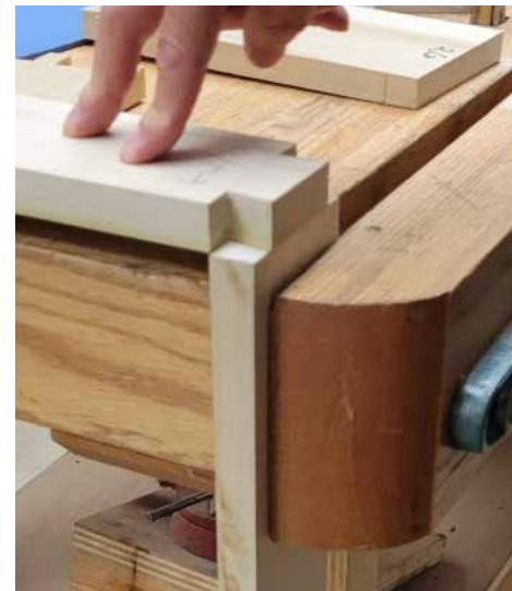
Use tail as template for pins
