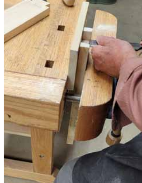
Cut lines perpendicular to bench top. Sit while chopping or sawing for tool stability. Note Chuck's hands holding his chisel.
