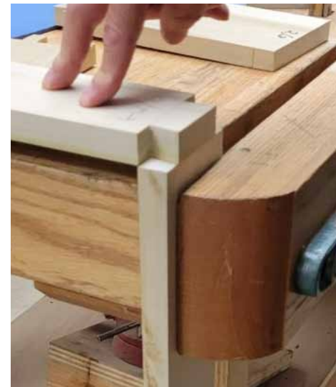
Use tail as template for pins
