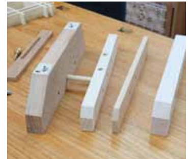
The jig disassembled to adjust widths \frac{1}{4} , \frac{1}{2} , \frac{3}{4} -inch-wide strips
