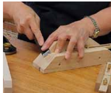
The jig for right-handed wood workers as the hand rests on the higher side.
