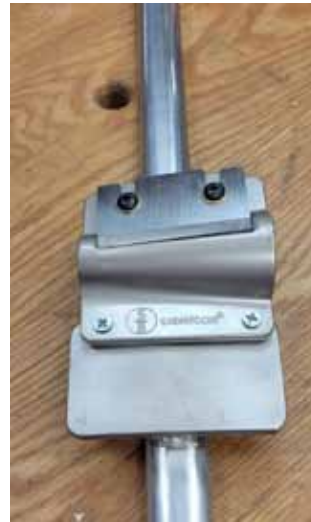
A special tool tapers and smooths one end of each leg
