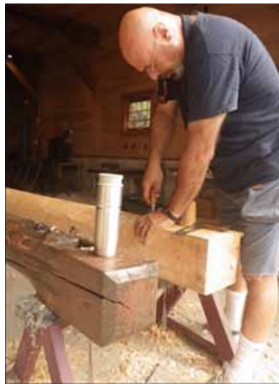
Shaping replacement mast
