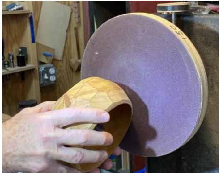
Stan sands a bowl on a sanding disk driven by a lathe.
