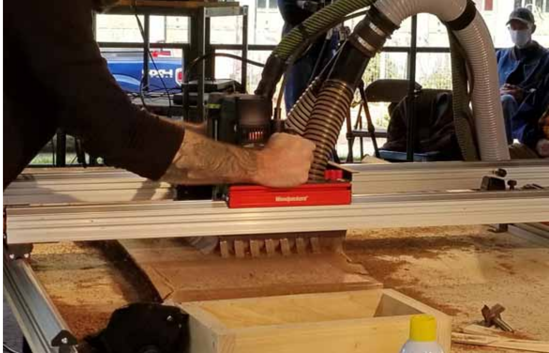
The slab flattening set up
