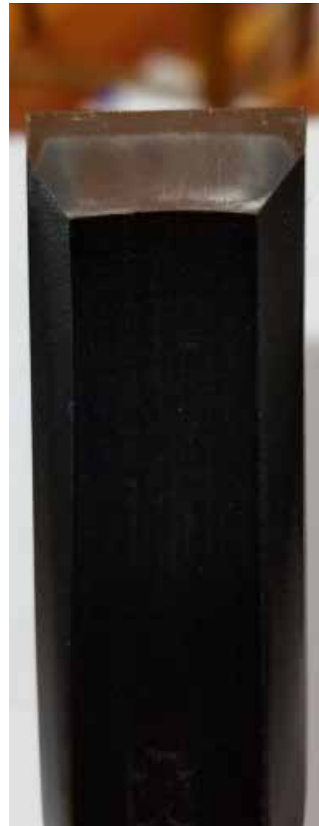
Japanese chisel has both hard and soft steel
