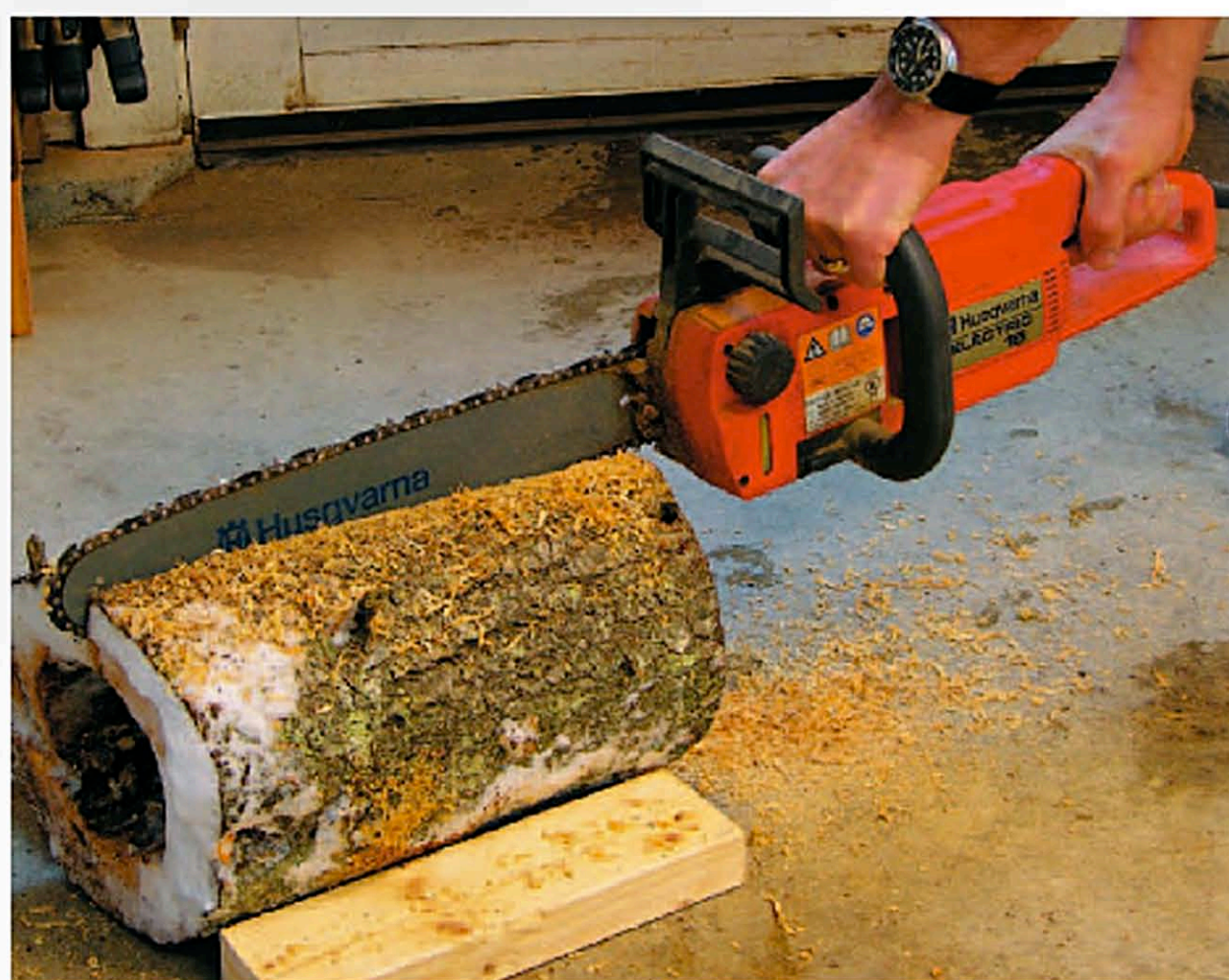
For a chainsaw ripping cut, note the blocks supporting the log. The shavings affirm that the blade is sharp.
