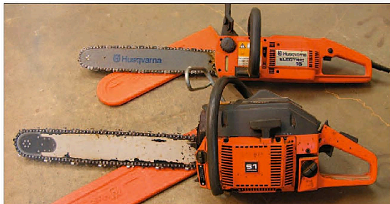
Two chainsaws appropriate for most woodturners: Electric with 16" bar (top) and gas powered with a 20" bar.
