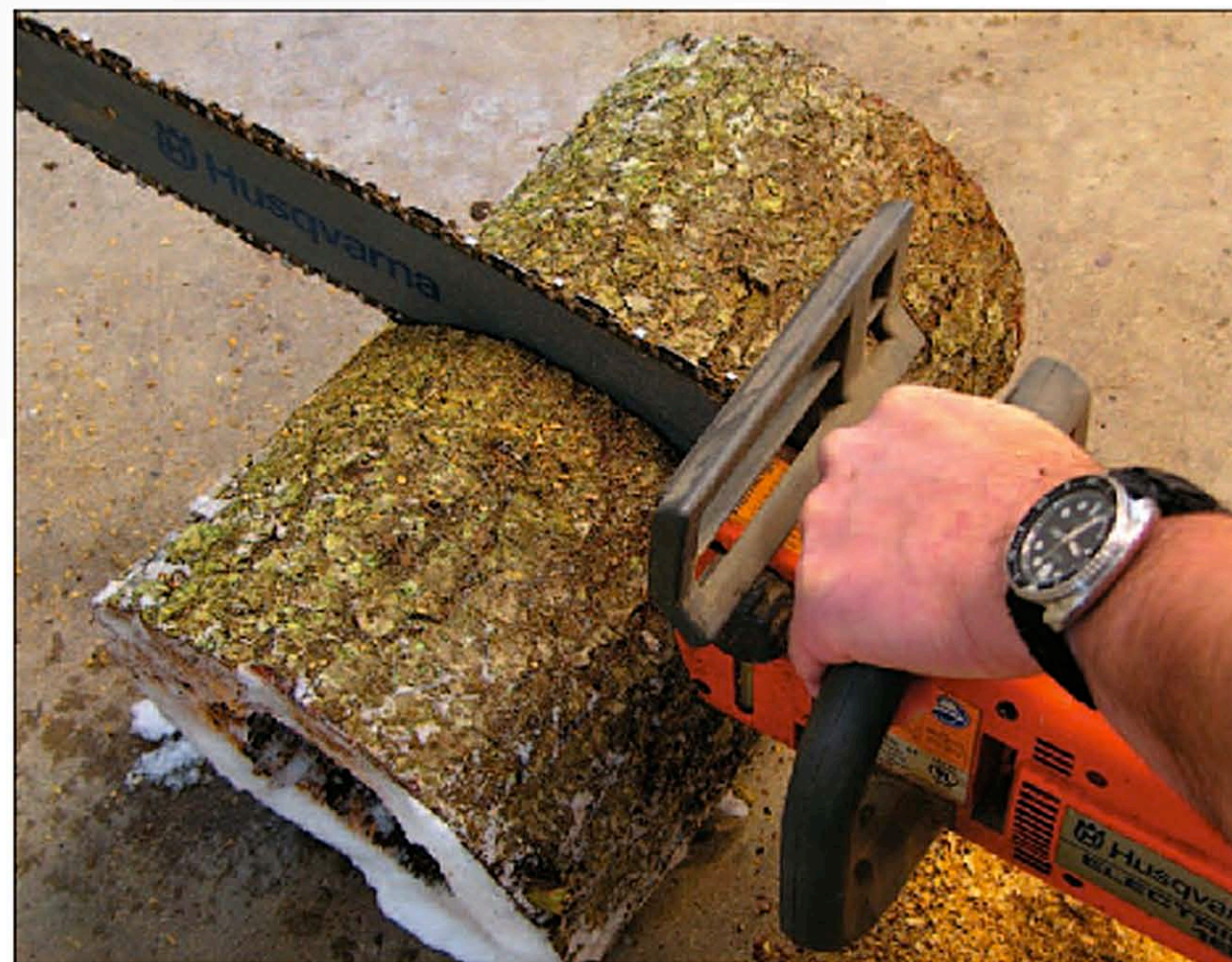
Every chainsaw task should begin with two hands on the machine. Note that the left hand is positioned directly in front of the chain brake on the handle.
