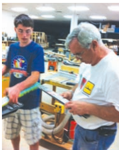
Matt countersinking mounting holes in skis
