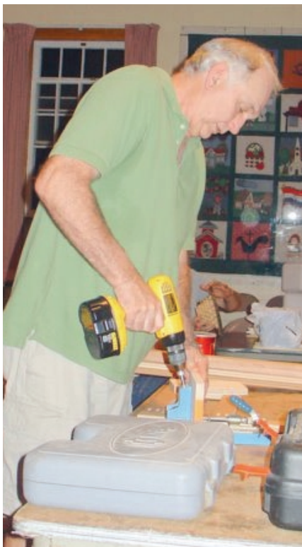
George drilling pilot hole using Kreg jig. All the components are stored in the case at bottom.
