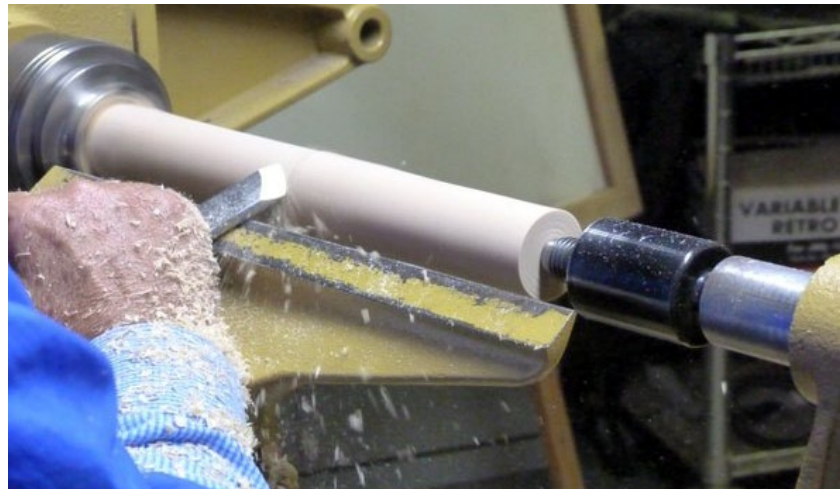
A radius skew is employed for a planing cut
