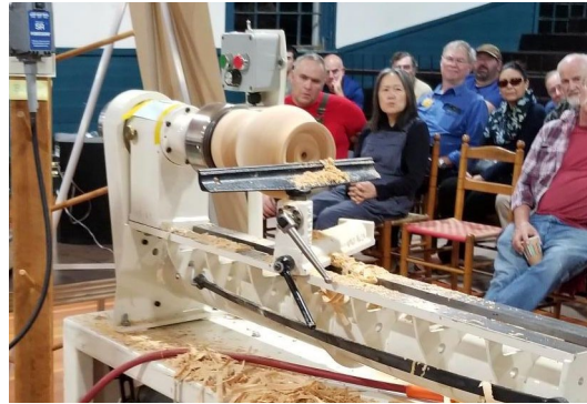
Starting the hollow cuts
