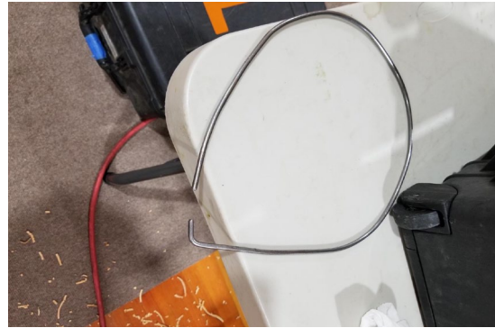
The flexible gauge to measure wall thickness
