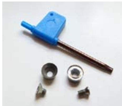
HSS cutter on left, carbide version on right. Note the carbide requires a longer screw. Both need Torx key.
