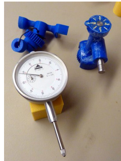
Examples of a runout gauge and thread chaser produced by Walt
