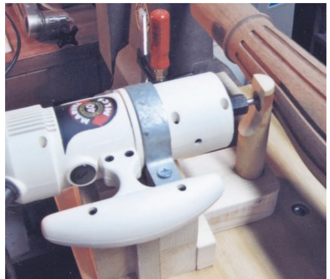
Ralph Zimmerman flutes a pedestal with is MLCS router sled.
