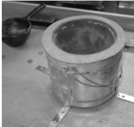
Flower pot furnace. Cast iron melting pot (crucible) left rear.
