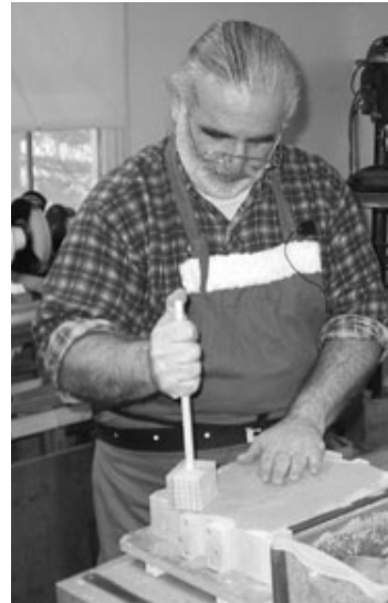
Ramming the sand to compact it and remove voids.
