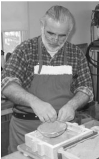
Michael Sofronas sifting sand over the pattern in the bottom of the flask (drag).
