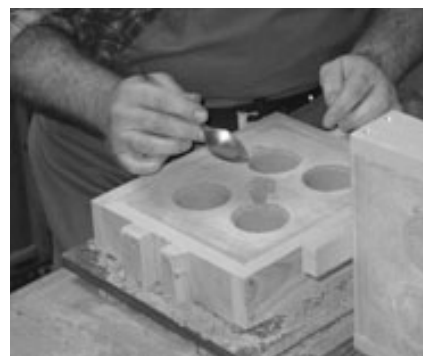
Forming gates for the metal to reach the mold cavity with a teaspoon.
