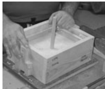
A dowel forms the opening (sprue) for the molten metal to enter.
