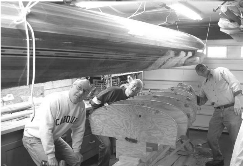
Hull raised off the forms, and the first look at the inside.
