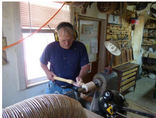
Frank Bondarenko roughs out a cylinder for an ornament
