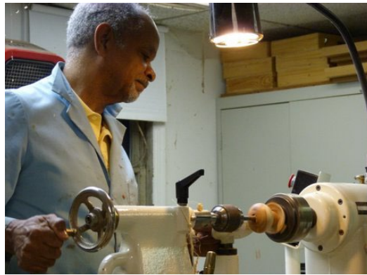
Matt drills a through hole in the ornament globe
