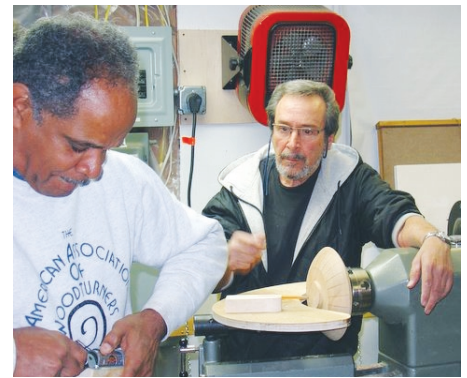
Matt and Steve demonstrating fluting technique. Note lathe mounted table for routing
