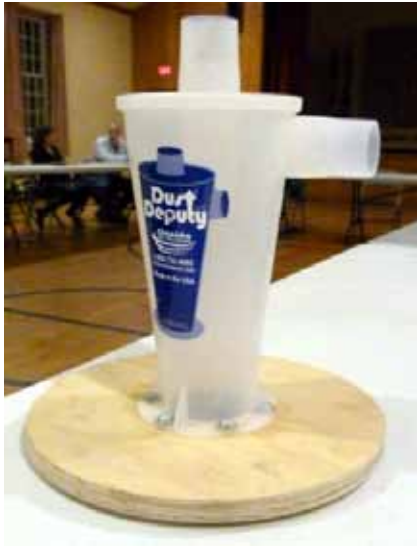
The Dust Deputy cyclone particle separator
