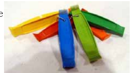
Fin combs are inexpensive tools to straighten dissipation vanes
