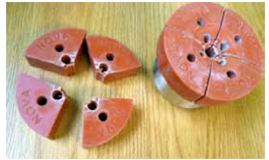
Nova soft jaws were used to turn small round jewelry pieces
