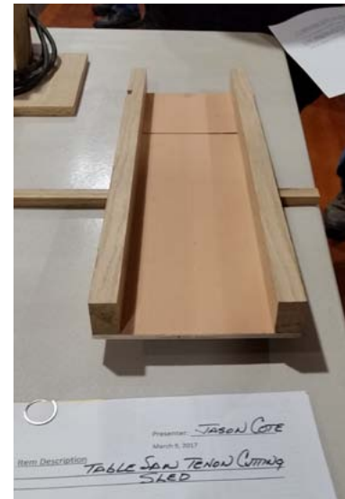
Tenon cutting sled - Jason Cotes
