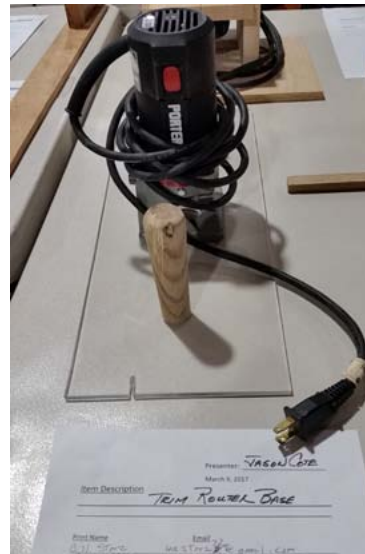
Plexiglass router mount - Jason Cotes
