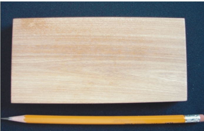
3" x 6" specimen of flat-sawn roble blanco wood.
