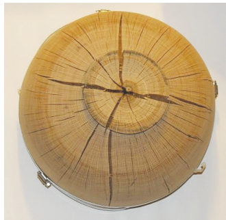
Oak bowl with severe cracks.
