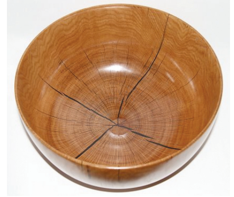
Finished bowl with the excess epoxy turned off.
