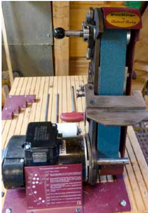
Sorby Pro Edge Sharpening Station is compact and features a groove in the platform to hold various jigs.
