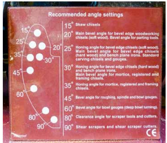
An angle guide on the front of the station lists the built-in settings.
