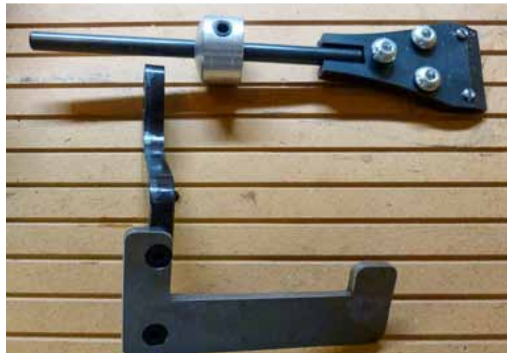
Other optional accessories include a jig for sharpening knives and a narrow platform for sharpening smaller tools.
