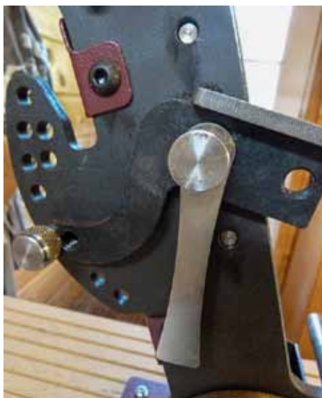
It's easy to set angles, using the selector on the side of the machine.
