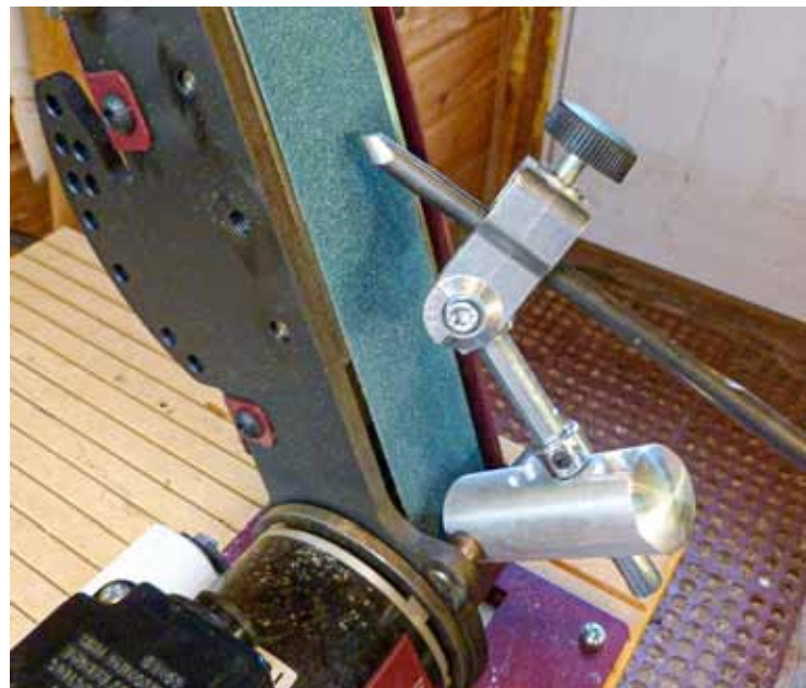
A "boss" can be used to fit a sharpening arm for parabolic profiles. The holes in the boss allow greater degrees of sweep back on the wings of the gouge.
